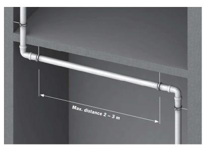
Horizontal pipework should be supported by pipe brackets in 3 meter intervals maximum. One bracket should be within 300 mm of the pipe joint and the other approximately at the midpoint of the pipe length, but not more than 3 metres from the next bracket (depending on the pipe diameter- refer to the upper table).
